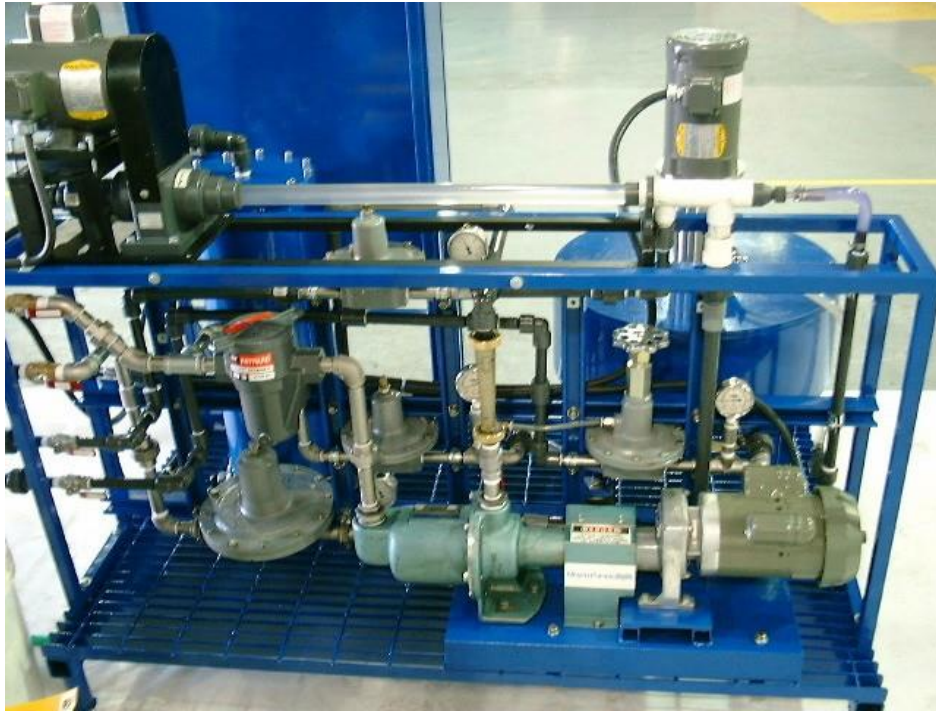
Example complete skid with three phase separator AVS 1000
